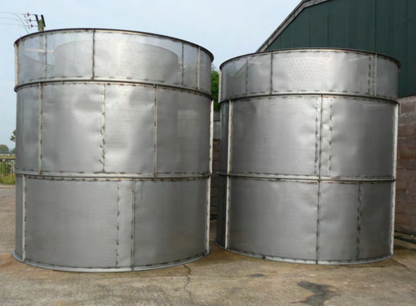
Adsorber internal cages prior to installation
